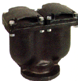
DOUBLE AIR RELIEF VALVE Body, bonnet: cast iron Floating balls: stainless steel Max rating temperature +80°C
